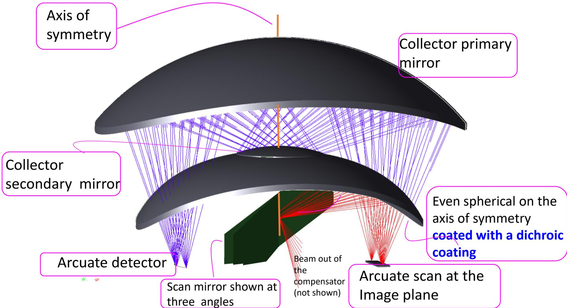
in TPM the scanning beam is usually in the IR, like 900nm (shown in red) and the collected light is at half the wavelength at 450 nm (shown in blue). The aspheric mirror is coated to reflect the long wavelength in the TPM case and transmit the short wavelength
